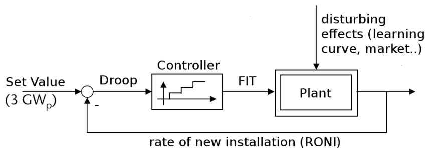
Fig 1: Sketched control scheme for PV FIT according to EEG 2012
